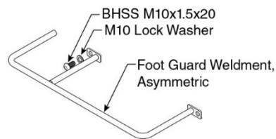
9/10AP Foot Guard Assembly, Asymmetric
