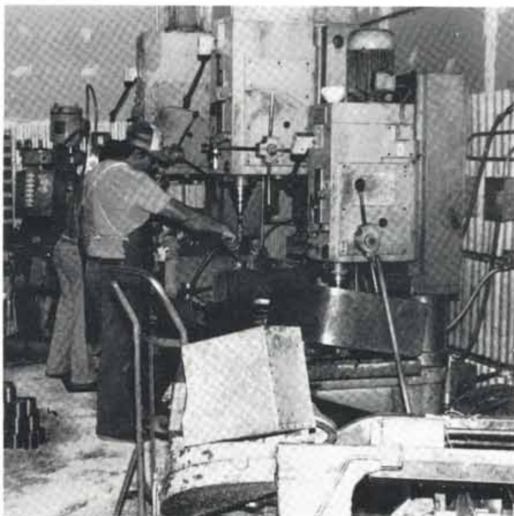
A Bend-Pak employee drills rounds for bender bumper ram dies.
