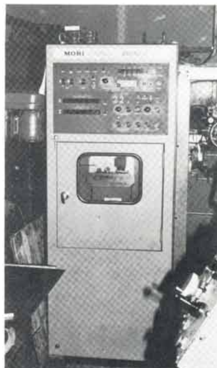
This unit is used to program Bend-Pak's die cutting lathes.
